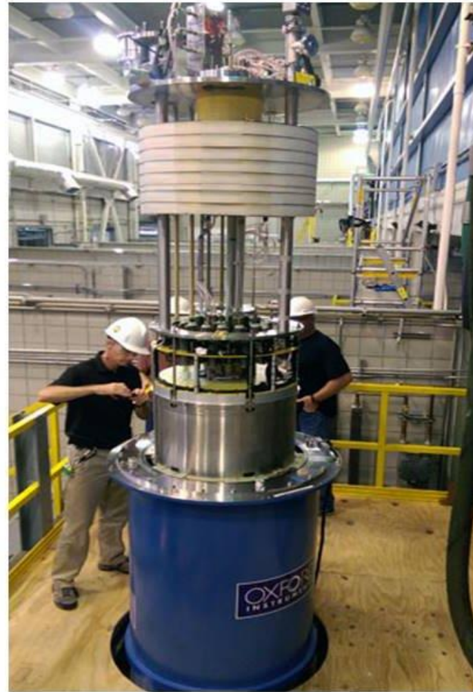
The 32 T is lowered into its cryostat, which keeps the instrument at a very cold operating temperature.
